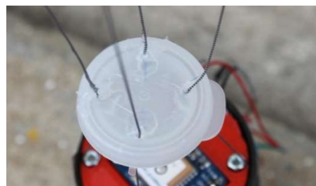
Fig. 4: the circular disk that prevents the cords from tangling
