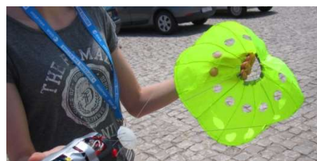
Fig. 3: the round canopy parachute
